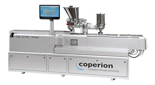
ZSK 32 Mc<sup>18</sup> smart with screw tip hight of 800 mm for easy accessability and electrical and water supply systems integrated in the baseframe. The Coperion K-Tron high-accurary feeders are mounted directly on the drive unit or if needed on the swivel arm of the ZS-B twin screw side feeder.
