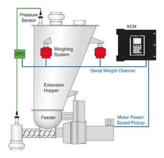
Basic principle of EPC electronic pressure compensation applied in gravimetric feeding system in a schematic presentation; KCM: feeding control
