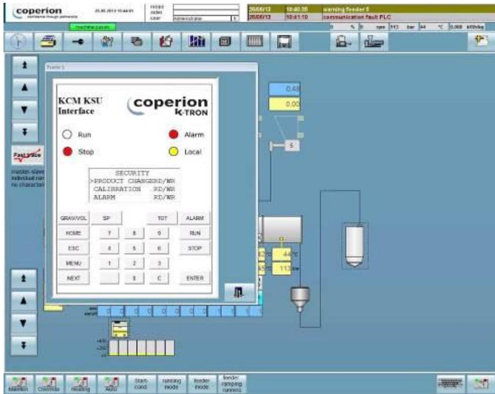
*The new CSpro extruder control system from Coperion permits central control and visualization of linked up feeding systems or other peripherals.*
