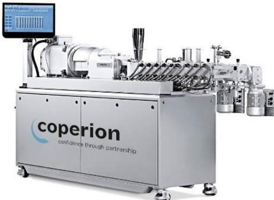
*The new ZSK 26 Mc<sup>18</sup> laboratory extruder from Coperion will be used by PolyOne specially for the development of polyamide compounds.*
