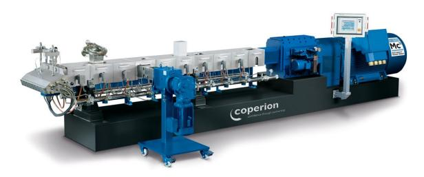
The new Coperion STS Mc<sup>11</sup> series with increased torque of 11.3 Nm/cm<sup>3</sup> is equipped with new Coperion-branded gearboxes from renowned European suppliers.
