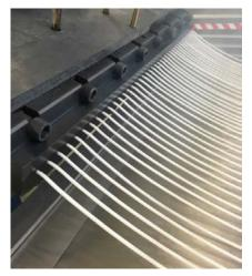
Coperion's new SK92 die head has been specially developed for high throughput rates.
