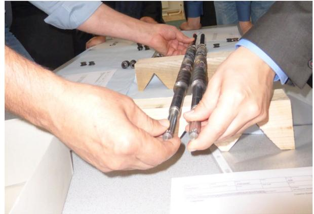
*The Food Extrusion Seminar 2015 at Coperion combined expert lectures (left) with practical demonstrations and exercises. Photo on right: Participants practicing screw configuration by “threading” various screw elements (conveying, mixing, shearing) onto the screw shafts.*
