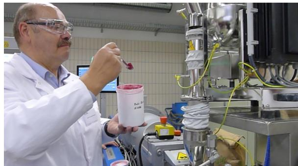
*ZSK 27 MEGAvolume PLUS with KT 20 feeder (Coperion K-Tron) fitted with cooling die (DIL). Practical demonstration: High-moisture extrusion cooking of newly developed meat analogues (photo left). Colored additives were used in order to visualize the process (photo right).*
