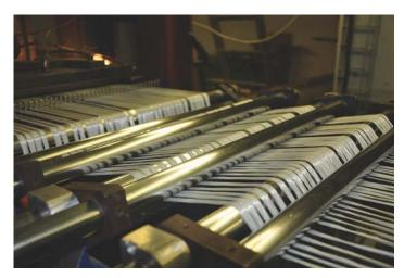
Roving pre-warming with spreading of the individual fibers enables the best individual fiber wetting.
