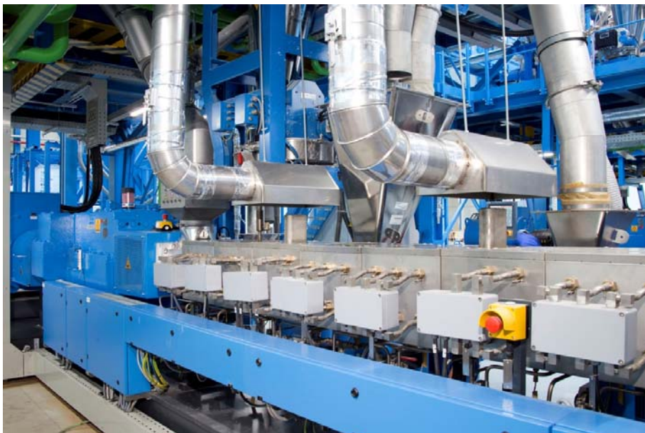
High-performance ZSK twin screw extruder for polyamide production
