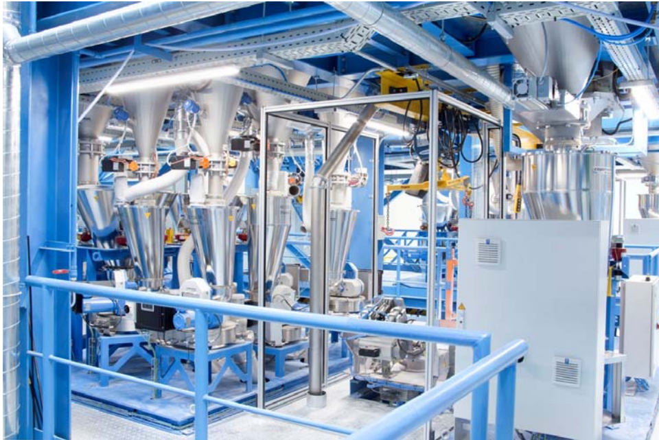
High-precision Coperion K-Tron loss-in-weight feeders
