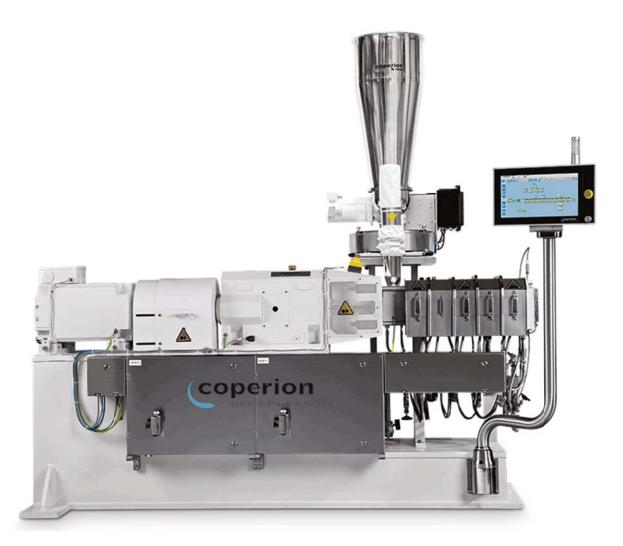
The ZSK Mv PLUS twin screw laboratory extruder offers ideal conditions for the extrusion of a variety of foods and pet foods.
