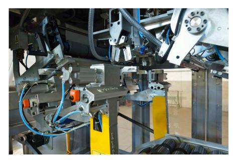
The FFS Packaging Machine ITL 500 with automated features provides accurate weighing, ideal dosing and hygienic packaging.
