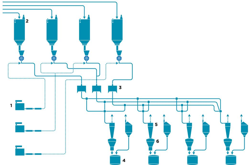
The systems engineers at Coperion K-Tron have extensive experience in handling and conveying even the most difficult materials. This process flow diagram illustrates a specialty material handling design which includes dehumidification systems for moisture-free conveying as well as in-line sifting and metal
