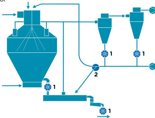
Coperion's hygienic design rotary valves and diverter valves are ideal for integration in sanitary conveying applications, such as spray drying of milk powders and infant formulas. Valve designs are available for discharge from spray towers, cyclones, sanitary receivers and for product line diversion to cooling operations, including complete CIP operation.
