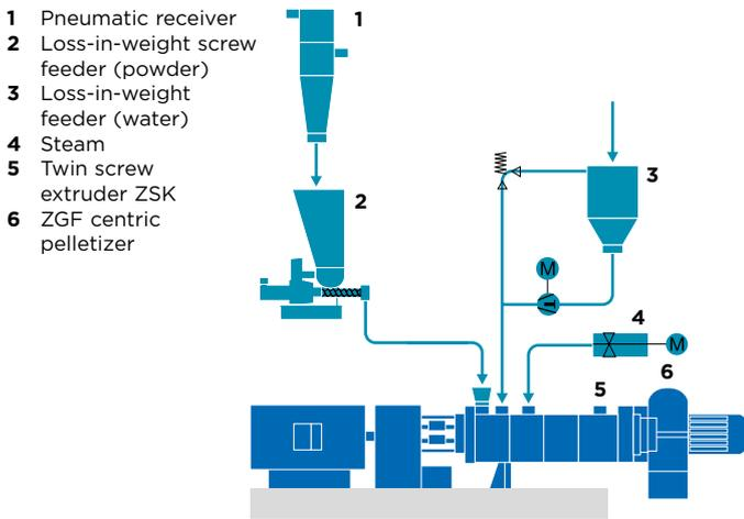
In comparison to conventional production methods of using a stirred kettle and roller dryer, production of flours and starches with a twin screw extruder has significant cost benefits. Excellent product feed characteristics allow the ZSK Mv PLUS to achieve very high throughputs even with small machine sizes. Investment and operating costs drop significantly compared to conventional production methods or to processes using older extruder series.
