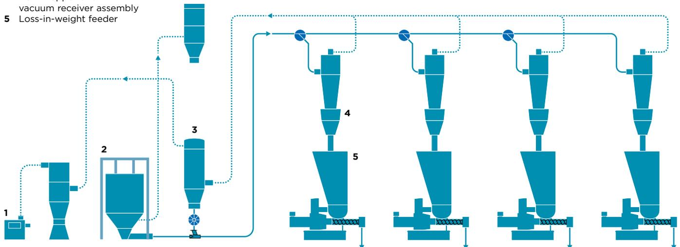
All continuous systems, whether for extrusion, mixing or coating, require accurate delivery of the product via loss-in-weight feeders, as well as continuous refill of the feeder hoppers. The
