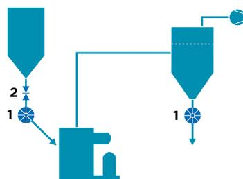
Coperion's PSR and ATEX rated rotary valves are ideal for integration into high pressure explosion protection milling systems for pressure isolation between the feeding mechanism and the product collector discharge point. They can also be used in conjunction with Coperion K-Tron screw feeders at the entrance of the milling system to ensure optimal and safe performance of the milling operation.
