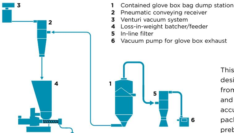
This specialty design material transfer line includes a custom designed glove box for optimal contained material transfer from bags directly to a Coperion K-Tron pneumatic receiver and loss-in-weight (LIW) feeder combination. The LIW feeder accurately batches micro-ingredients direct to the supersack packaging line. Ideal applications are handling of probiotics, prebiotics and vitamins.
