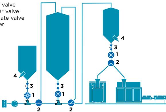
Coperion's reliable rotary valves are the right choice for the discharge of powder and granules out of silos and hoppers into dilute phase or dense phase pneumatic conveying systems. They ensure highest conveying capacities. Coperion's rigid diverter valves enable safe routing of products to several directions.
