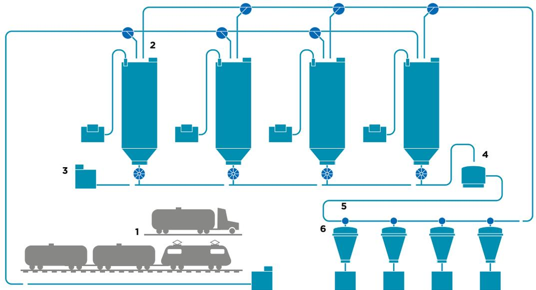
The systems engineers at Coperion K-Tron can help design the optimal ingredient transfer system for your operation, such as moving flour, starch, or sugars from railcars, trucks or bulk bags to the process. Flow diagram above illustrates PD rail unloading
