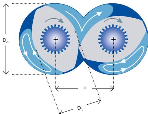
$D_o$  = outer diameter |  $D_i$  = inner diameter |  $a$  = center line distance |  $D_o/D_i$  = outer/inner diameter ratio, determines shear and free volume |  $Md/a^3$  = specific torque, determines output density and degree of fill |  $n$  = screw speed, determines shearing and mixing
