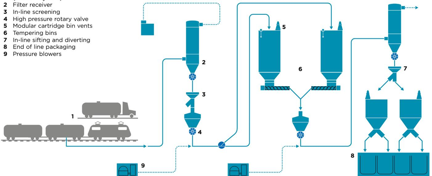
Coperion provides dense phase conveying systems for even the most fragile materials. The system shown illustrates rail and truck unloading of corn grits directly to a filter receiver, with in-line sifting prior to entrance to a dense phase positive
