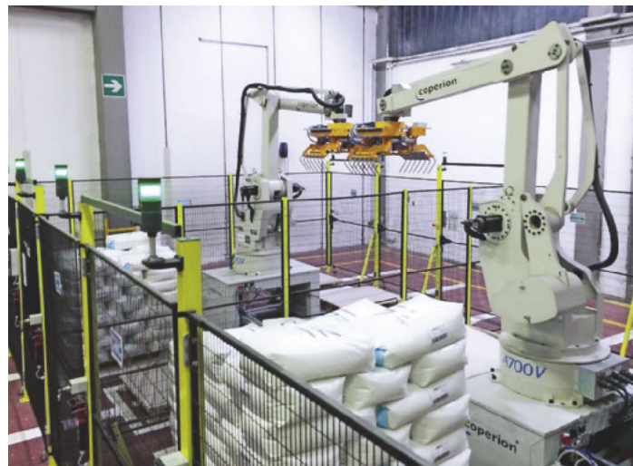
The palletising island is equipped with two four-axis robots which stack the filled bags in 12 palletising positions
