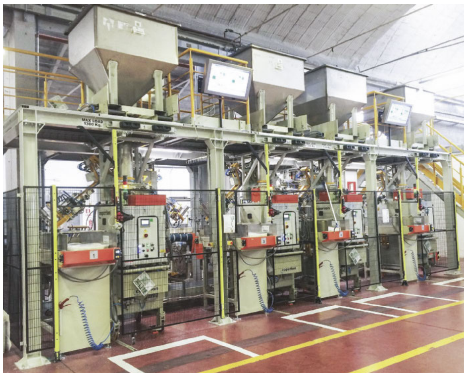
Sabic Italy installed six Coperion packaging lines and a common palletising island at its plant in Pontirolo
