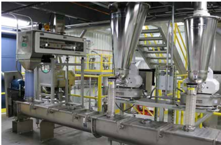
► Coperion K-Tron Smart Weigh Belt Feeder metering peanuts into screw conveyor and LIW Twin Screw Feeders dosing ingredients into nut mixture. Source: Coperion K-Tron.
