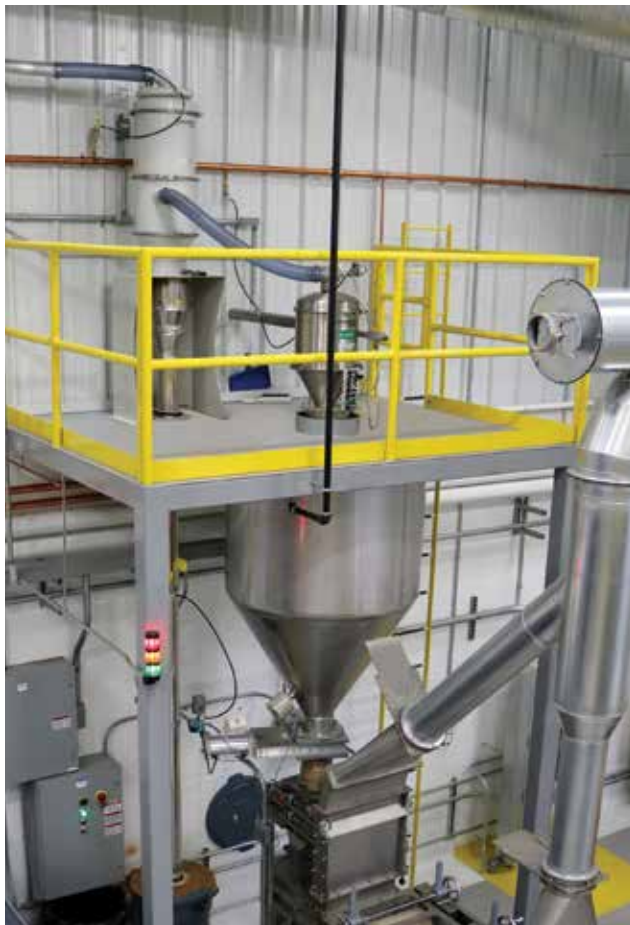
► A Coperion K-Tron 2400 vacuum sequencing receiver with an inline filter conveys roasted peanuts to the blancher. Source: Coperion K-Tron.
