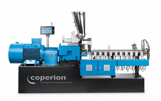
Coperion's twin screw extruder STS Mc<sup>11</sup> has a specific torque of 11.3 Nm/cm<sup>3</sup> and features up to 27% higher throughput rates than the preceding model.
