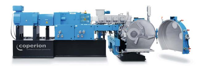
Coperion's Kombiplast KP two-stage processing system, equipped with EGR eccentric pelletizer and the new knife rotor (patent pending), for the production of enhanced quality PVC pellets.
