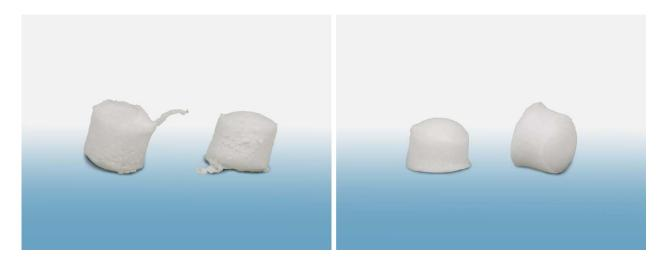
In contrast to conventional knife rotors (left), Coperion's new EGR knife rotor obviously minimizes dust content of PVC pellets(right).
