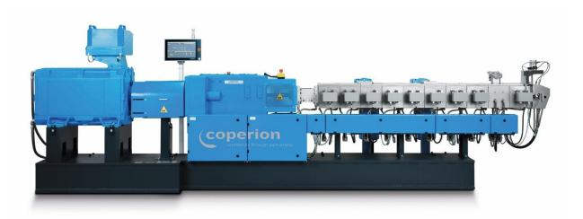
The ZSK 58 Mc<sup>18</sup> world proven twin screw extruder is a best-practice design of the Coperion ZSK extruder, and is ideally suited to compounding all engineering plastics.
