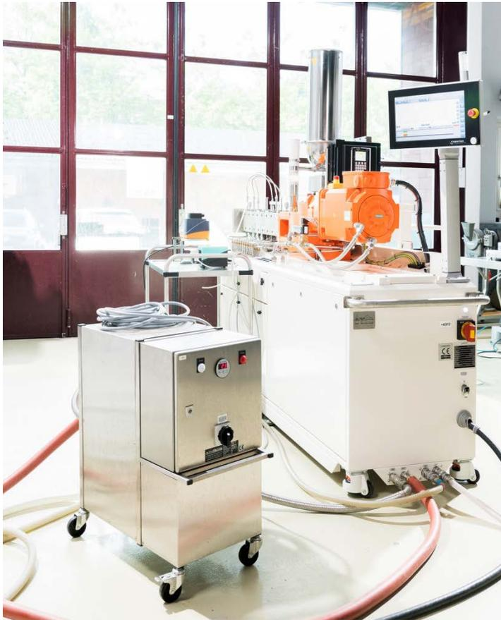
*The Coperion food extruder ZSK 27 Mv PLUS is equipped it with many quick-change features and devices for flexible processing set-up to allow the Zurich University of Applied Sciences to use the extruder for a wide variety of research and development work.*
