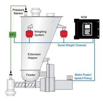
Basic principle of EPC electronic pressure compensation applied in gravimetric feeding system in a schematic presentation; KCM: feeding control
