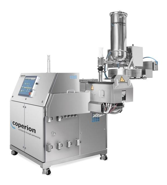
Coperion's ZSK 18 MEGAlab twin screw extruder with Coperion K-Tron gravimetric loss-inweight feeder, suitable for research and development as well as for small-scale production
