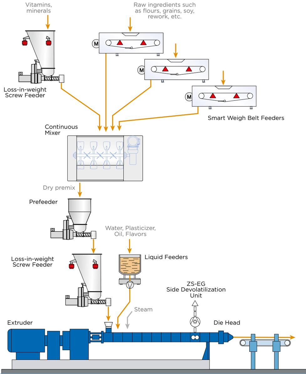
extruder with the highest free volume on the market. This enables our customers to run higher throughputs than on other machines with similar screw diameters.
