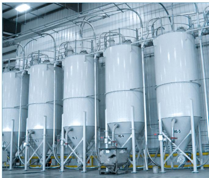
Coperion K-Tron pneumatic conveying system
