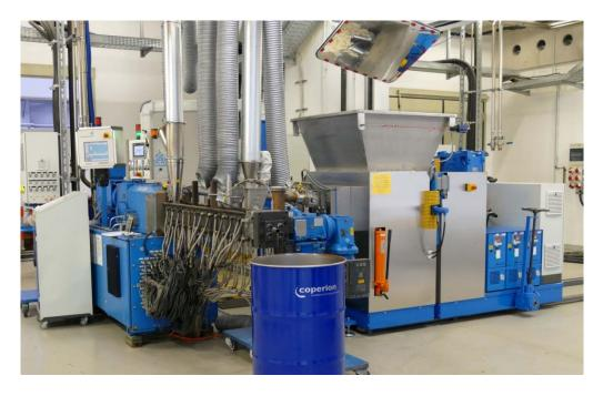
Setup for a live demonstration for HMPSA (Hot Melt Pressure Sensitive Adhesives) production with a ZSK 34 Mv PLUS twin screw extruder from Coperion and a Roll-ex system for feeding rubber bales into the extruder.
