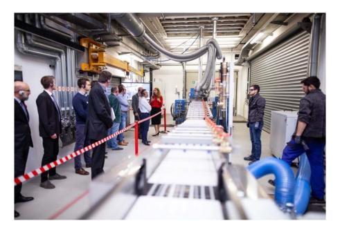
Setup for a live demonstration of anti-block masterbatch production with Coperion's ZSK 58  $Mc^{18}$  twin screw extruder, its patented Feed Enhancement Technology (FET) and a semiautomatic SCP strand conveyance unit SCP.
