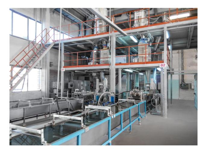
R&P POLYPLASTIC produces mainly polypropylene, polyamide, and polyethylene compounds for processing into auto parts, household appliances and construction materials on STS 75-type twin screw extruders from Coperion.
