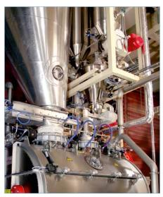
Coperion K-Tron screw feeders in a vacuum coating process
