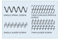
Figure 4 - Basic single and twin screw geometries
