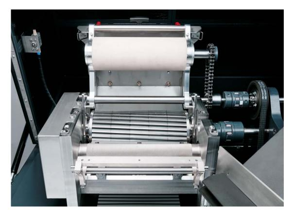
The SP 240 strand pelletizer is equipped with a new cutting gap adjustment technology that enables faster and more comfortable adjustment.
