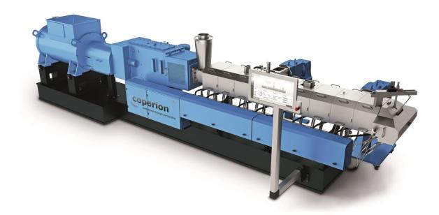
Within the ZSK Mc<sup>18</sup> twin screw extruder, shredded production waste is processed such that it can be added back into the multi-layer film production process — at consistently high end product quality.
