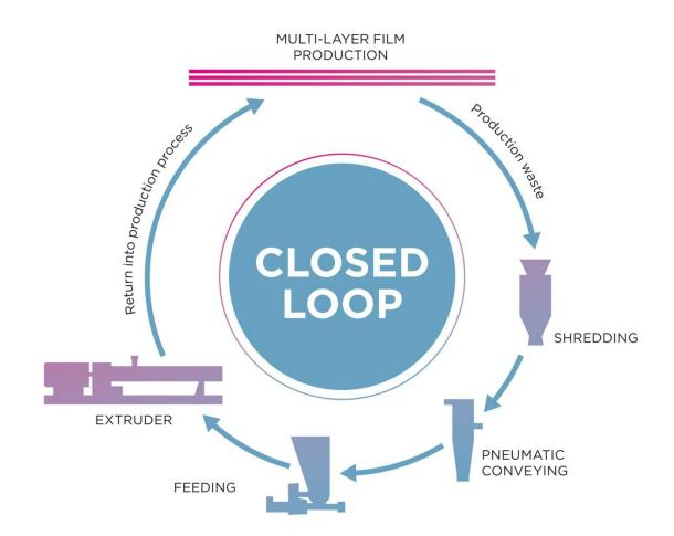
With Coperion's innovative closed-loop approach, production waste resulting from multi-layer film production can be re-added and re-processed within the manufacturing process at a rate of up to 100%.
