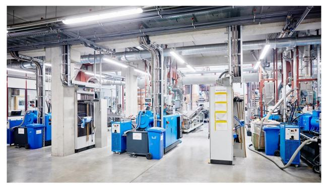
Aurora's new production area is equipped with ultramodern ZSK 45 compounding systems from Coperion.
