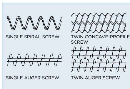
Figure 4 - Basic single and twin screw geometries
