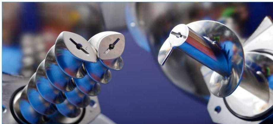
Figure 1: Twin and single screw feeders are used for a wide variety of raw materials
