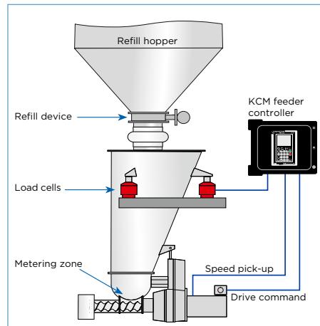
Figure 3 - Gravimetric loss-in-weight (LIW) feeder principle: A loss-in-weight (LIW) feeder is a gravimetric feeder that directly measures the material's weight to achieve and maintain a pre-determined feedrate that's measured in units of weight per time.
