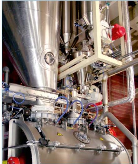
Coperion K-Tron screw feeders in a vacuum coating process
