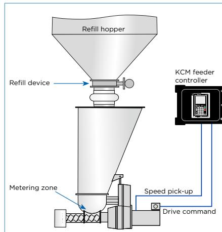
Figure 2 - Volumetric feeder principle: A volumetric screw feeder feeds a certain material volume per unit time to a process.
