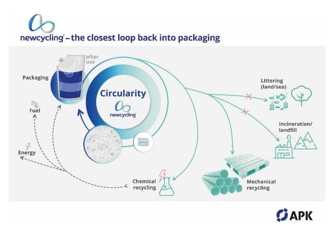
Unique plastic recycling technology Newcycling<sup>®</sup> from APK that manufactures clean, singleorigin PA and PE pellets out of complex PA/PE multi-layer film waste, with properties similar to virgin product.
