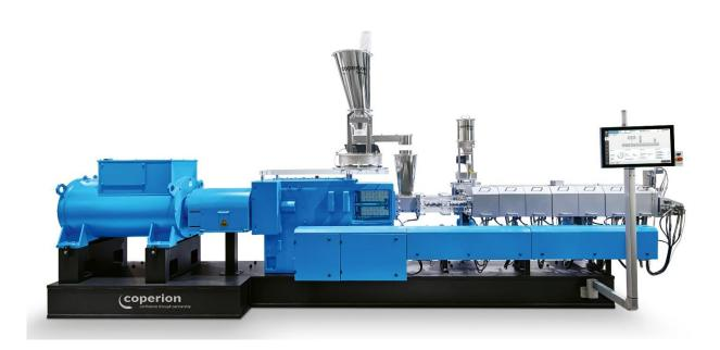
ZSK twin screw extruders from Coperion are ideally suited for APK's Newcycling<sup>®</sup> process due to their high dispersion and degassing performance.
