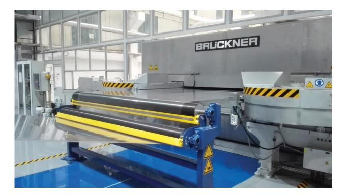
Plastic film stretching line from Brückner Maschinenbau, in which ZSK extruders from Coperion take over the melting of the compounds.
