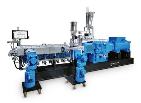
In this project, addition of fillers to the polymer in the Coperion ZSK twin screw extruder is being improved to avoid creating agglomerates and degrading the polymer during compounding.
