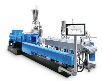
The ZSK 70 Mc<sup>18</sup> twin screw extruder has a screw diameter of 70mm and incorporates numerous features, which improve handling and increase efficiency in compounding and recycling.
