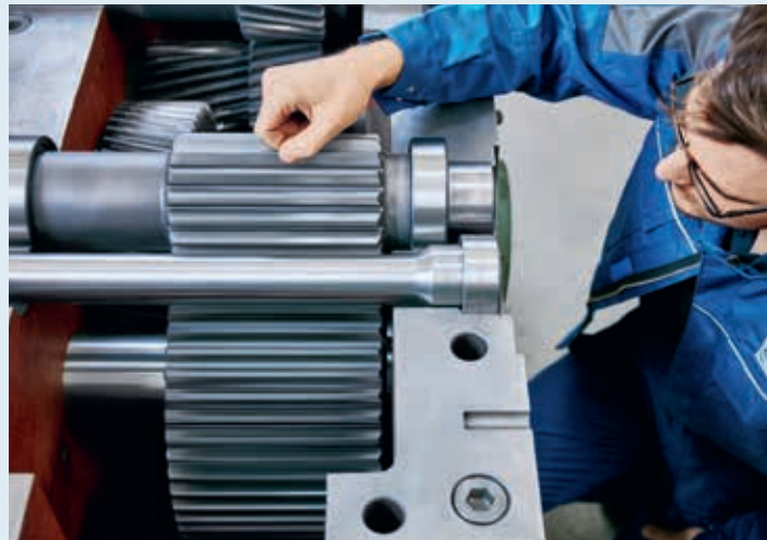
› CLEARANCE CHECK OF GEARBOXES
