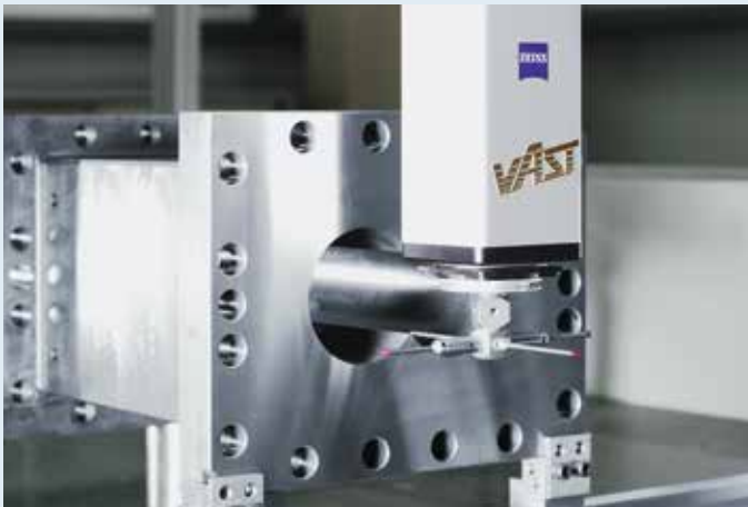
› 3-DIMENSIONAL BARREL INSPECTION CENTER
