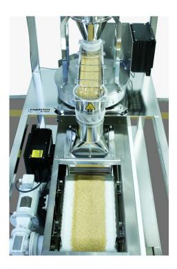
Coperion K-Tron's newest generation of loss-in-weight feeders with vibratory trays enables gentle bulk material handling, higher feeding accuracy, and shorter changeover times.
