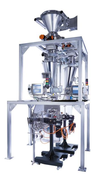
Compact size is one feature of the Coperion ZSK 26 Mc<sup>18</sup> laboratory extruder with Coperion K-Tron feeders for recipe development and validation.
