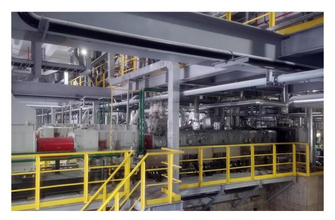
Coperion's ZSK Mc<sup>18</sup> twin screw extruder is playing a key central role in this system for particularly energy-efficient manufacturing of acrylonitrile-butadiene-styrene copolymer (ABS) blends.
