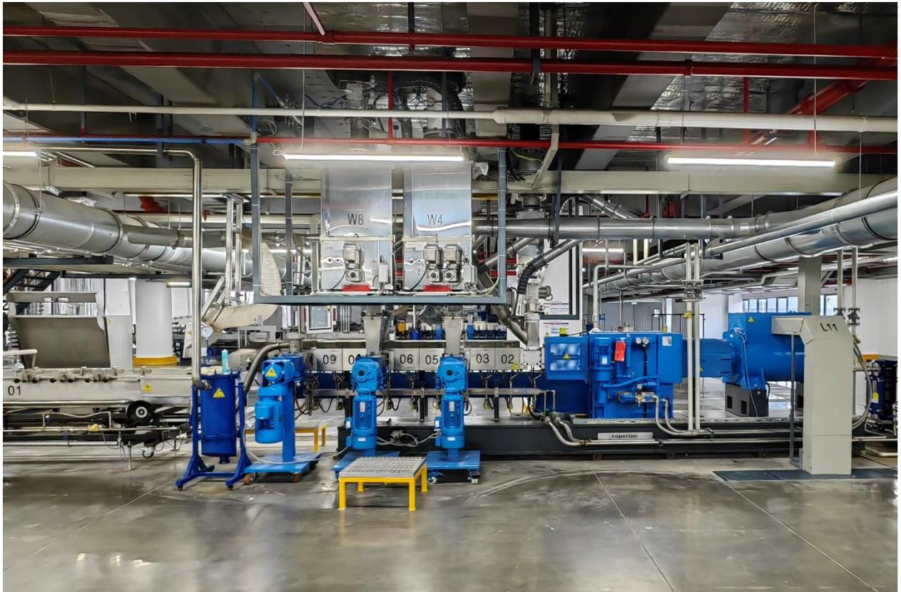
Chuanghe has acquired four of Coperion's high-performance ZSK Mc<sup>18</sup> twin screw extruders.
