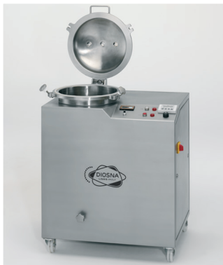
Explosion-protected mobile liquid preparation vessel with stirrer, and with integrated control.
