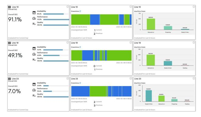
With C-BEYOND, important ZSK extruder performance markers, such as availability, production quantity and product quality, are determined in real time and visualized in user-friendly OEE analysis diagrams.
