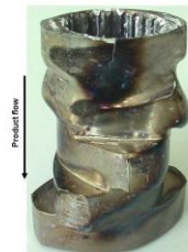
Excessive wear due to abrasive materials
